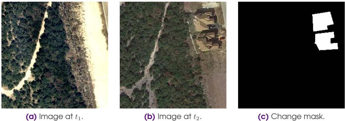
Figure 1: Example bitemporal LEVIR-CD patch used in the experimental pipeline. The model receives the two RGB images and predicts the binary building-change mask. Additional qualitative outputs are reported in Appendix C.
